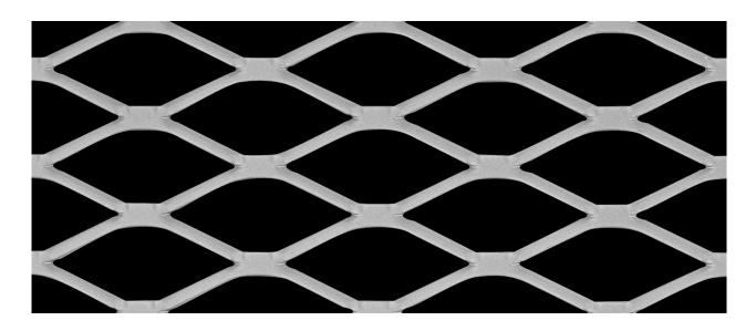
LW Aperture: 43.18mm Strand Width: 3.23mm SW Aperture: 17.27mm Thickness: 1.50mm Weight: 3.24 kg / m2 Open Area: 73%
